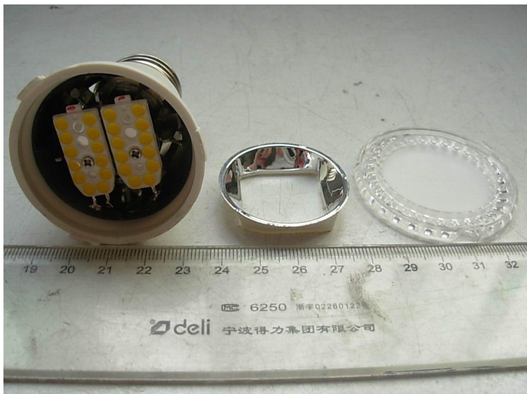
FIGURE 8. LED SPOT LIGHT (M/N: 50-45EUS) COVER REMOVED
